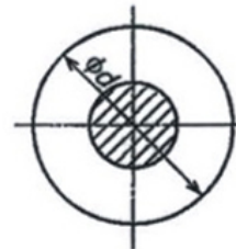
b) Round bar test piece where d \leq 25 mm
